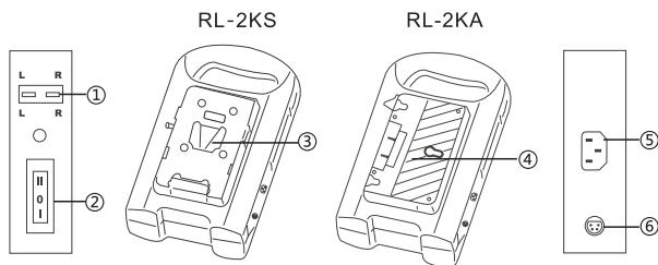
① Charging indicators    ② Function switch button    ③ V-Mount plate
